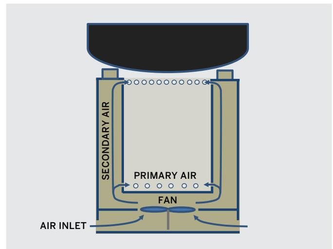
airflow. To address this challenge, forced-draft stoves use a fan or blower to control primary and secondary air, making the air flow more predictable and adjustable.
