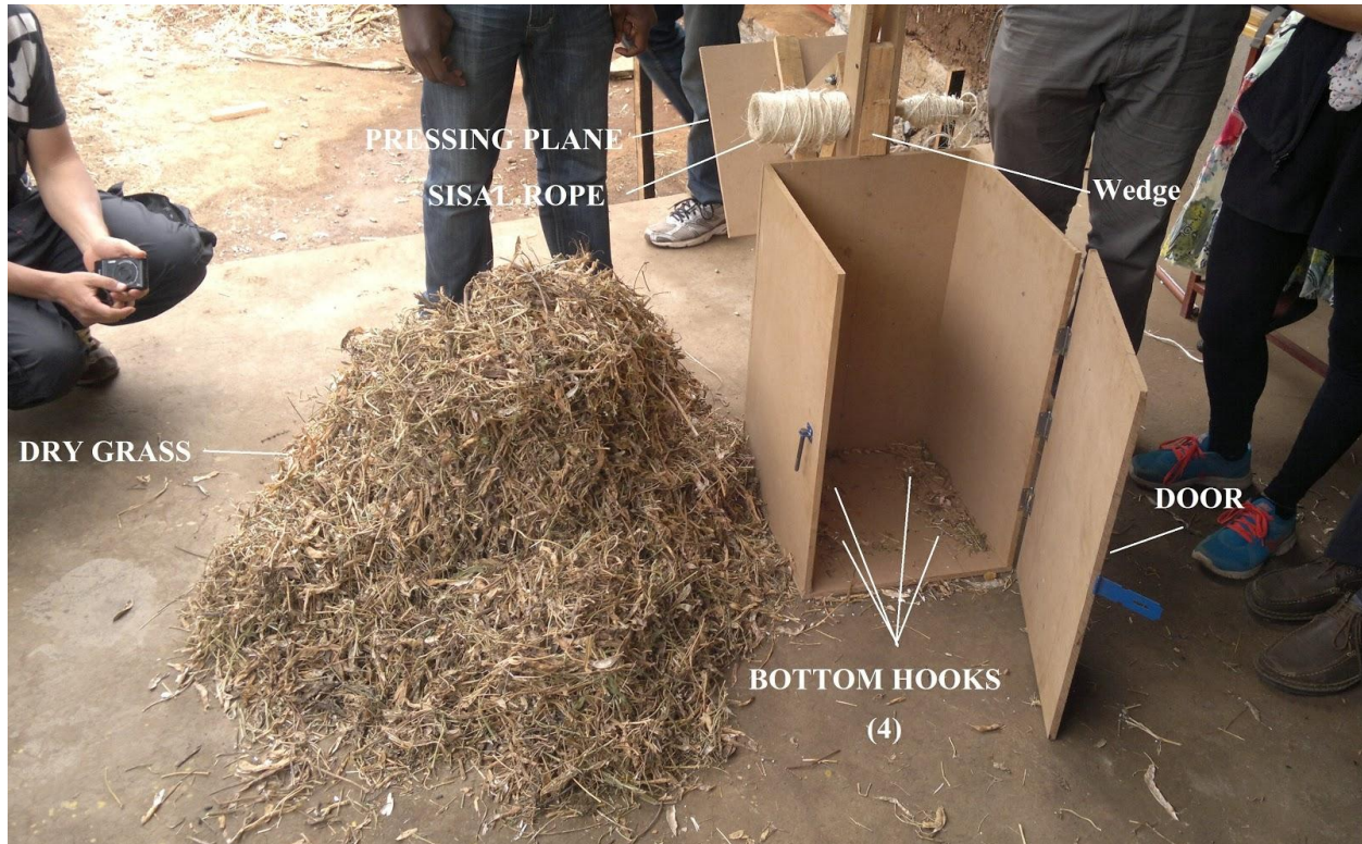
Fig. 11 Important baler components
