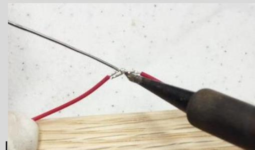
Always put the solder on the component, not directly on the soldering iron, as this will cause more solder to be burned without actually attaching anything. You want to see the solder glide quickly across the metal.
