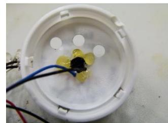
17. The LEDs will press-fit into the drilled holes. Line the tip of the LED up with the hole and press gently until the LED is fit snugly in the hole.
