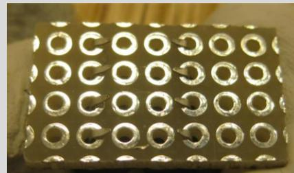
Apply the right amount of solder. Using the 4-second rule, solder the component to the metallic ring that it comes out of on the circuit board. Apply just enough solder to fill the hole. If connecting two things on the circuit board, solder the second component to the metallic ring first. Then, touch the soldering iron to the portion of the second component resting on the already soldered component. This will re-melt the area and allow the components to connect.
