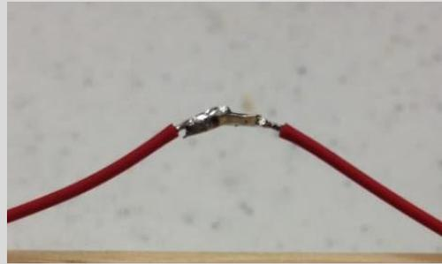
*Avoid overheating.* Make sure to not leave the soldering iron tip on any one component for too long, as it can burn components and cause them to stop functioning. If something still isn't attached after the four second rule, stop, allow the components to cool down, and begin again. All of the components are susceptible to intense heat, so be careful not to overheat them. The battery packs in particular are very easy to melt, so follow the four second rule closely.
