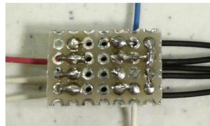
Solder each of the wires to its corresponding pin.
