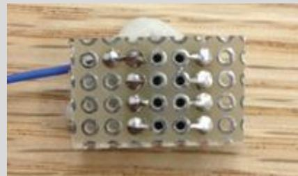
If your soldered connections are overlapping in places that aren't supposed to be connected, you probably applied too much solder and the circuit will short.
