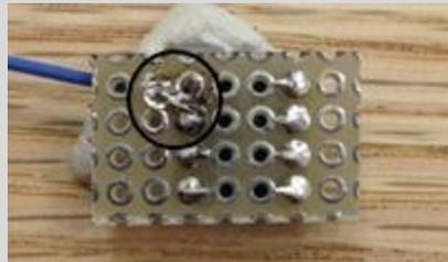
10. Turn the board, with the socket soldered on, back over. The pins of the microcontroller are numbered counterclockwise from the top left. No wires will be connected to pins 1 and 6.
