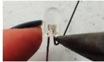
2. Strip a piece of wire selected for 'ground' and a piece of wire selected for 'current'. Twist the multi-stranded wire so that the strands have more physical integrity. Bend the stripped ends of these wires into u-shapes and connect them with the u-shaped bends made on the LED.
