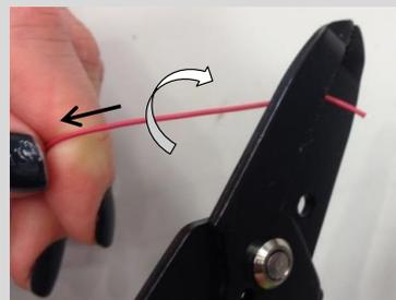
*Check the result.* Your resulting wire should look clean, as in the figure to the right. Be careful not to cut the inside silver wire or any of the individual strands of silver wire if you are using stranded wire. This happens when you use too small of a gauge. If you use too large of a gauge, the colored casing will not be cut all the way through. When in doubt, cut away the stripped wire and try again
