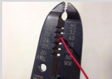
*Strip the wire.* Using your free hand, twirl the wire in a few circles while tugging gently until the colored casing has become separated from the silver wire inside. Continue to pull on the wire until it has been stripped.
