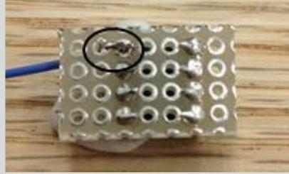
If the metallic holes aren't filled with solder, and you can wiggle your wires loose, you probably haven't applied enough solder.
