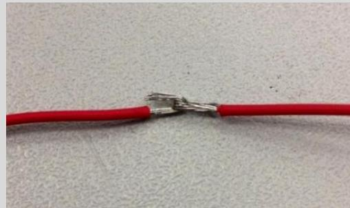
*Apply solder.* Solder is like metal “glue.” Just as with normal glue, you do not need to use a lot to get things to stick. The soldering process should only take 4 seconds. Think of it this way:
