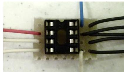
12. With the wires in place, turn the circuit board over and secure it to the putty and block. This can be done after all of the wires are in place or one at a time. Bend the ends of the wires to touch the pins they correspond to. With the grounded wires, bend first the end of the wire that is closest to pin 7 to touch the pin, then bend the other grounded wires to connect to each other in the black "T" shape shown in the figure.
