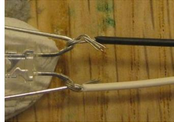
*Teaching note: Explain that in building a circuit, it helps to keep all of the ground wires consistently one color while the current wires are consistently a different color.*
