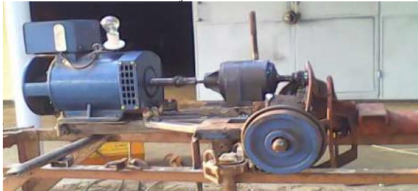
Figure 1: generator assembly attached to a step-up gear at workshop.
