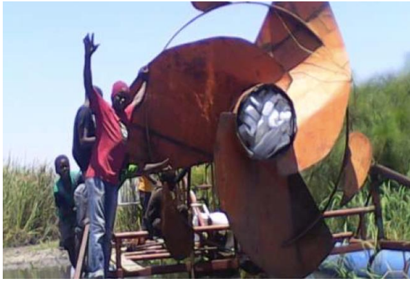
The picture below shows the actual turbine on the testing site on the Kafue River, raising his hand is Robert Shimaingo
