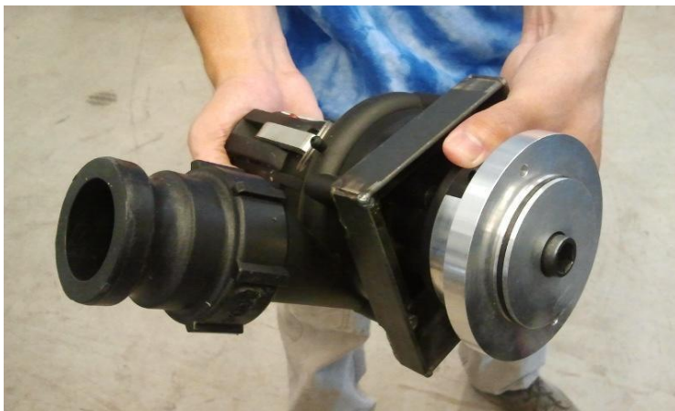
Booster Pump Assembly.
