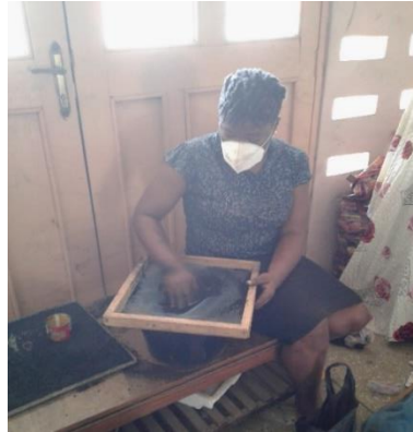
PLATE 3.8: SIEVING OF THE CRUSHED COCONUT HUSK
