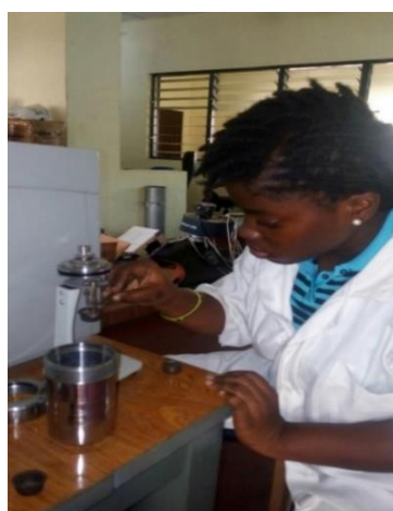
Plate 3.23: Winding of The Firing Wire On the Electrode Rods
