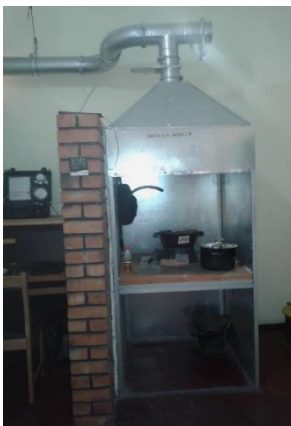
Plate 3.25 Section of The Laboratory Emission Monitoring System
