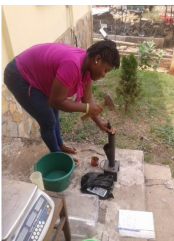
Plate 3.13: Hammering Of The Plunger To Make The Briquette Compact
