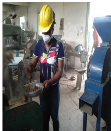
PLATE 3.11: FEEDING OF CHOPPED COCONUT HUSK INTO HAMMER MILL
