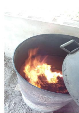
PLATE 3.3: THE INITIAL CHARRING PROCESS
