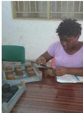
Plate 3.17: Determining The Length Of Uncharred Briquette Using A Digital Vernier Calliper
