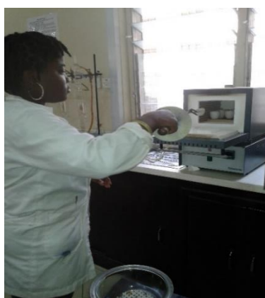
Plate 3.20: Researcher Transferring Samples Into The Furnace
