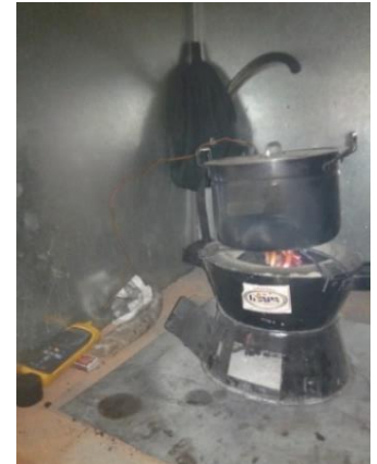
Plate 3.28: Ongoing Water Boiling Test
