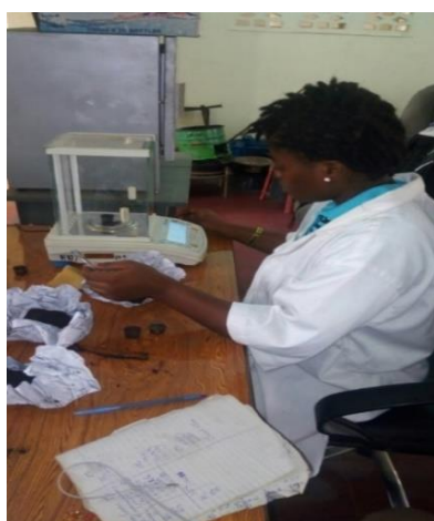
Plate 3.22: Weighing of Pulverised Briquettes Using an Analytical Balance
