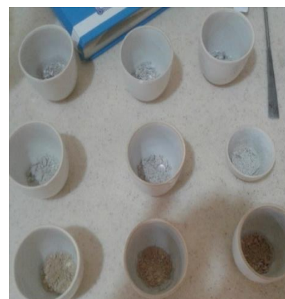
Plate 3.21: Samples Of The Fragmented Briquettes After Removal From The Furnace
