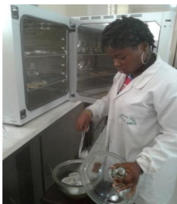
Plate 3.19: Transferring Of Fragmented Briquettes Into The Oven
