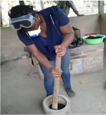
PLATE 3.7: CRUSHING OF THE CHARRED HUSK
