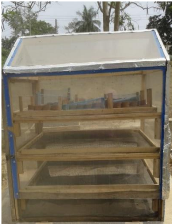
Plate 3.16: Drying Of The Briquettes In The Solar Drier
