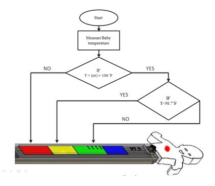
The microcontroller is programmed using Arduino open source software. The analog output of the temperature-measuring sensor is given to microcontroller port  $A_0$ . The HIGH or LOW output of the
