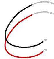
Each wire should have one side that is stripped 4" and the other side with 1" stripped.
